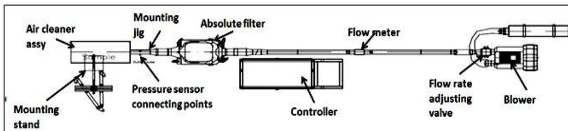
Figure 3 Air filter test set up
