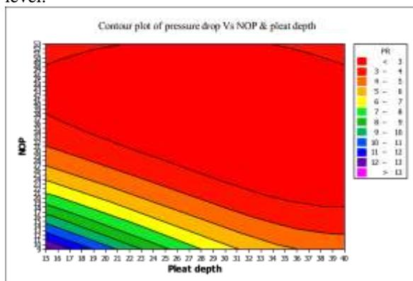
Figure 10 Contour plot of PD vs. NOP & pleat depth
