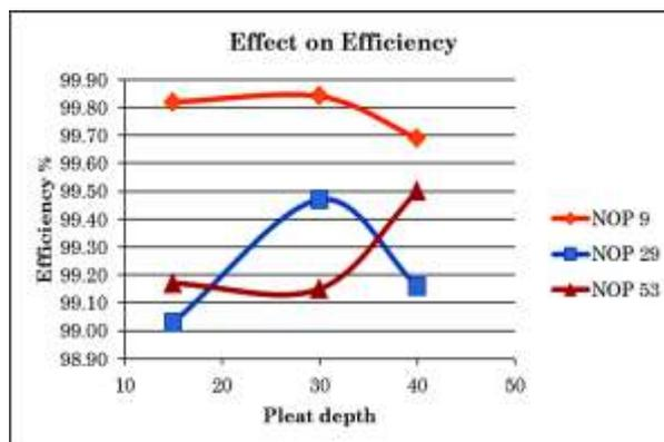
Figure 6 Effect of pleat depth on efficiency
