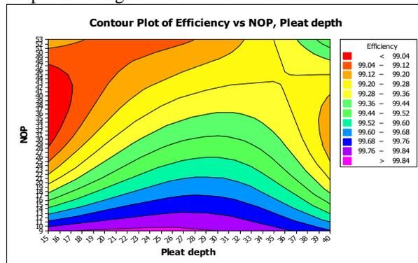
Figure 12 Effect of efficiency vs. NOP & pleat depth
