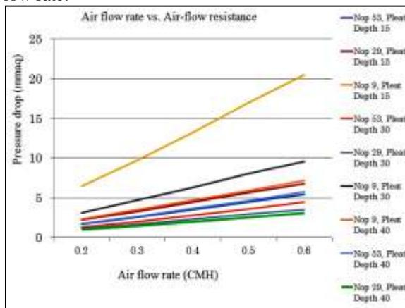
Figure 15 Graph plot of pressure drop vs. air flow rate.
