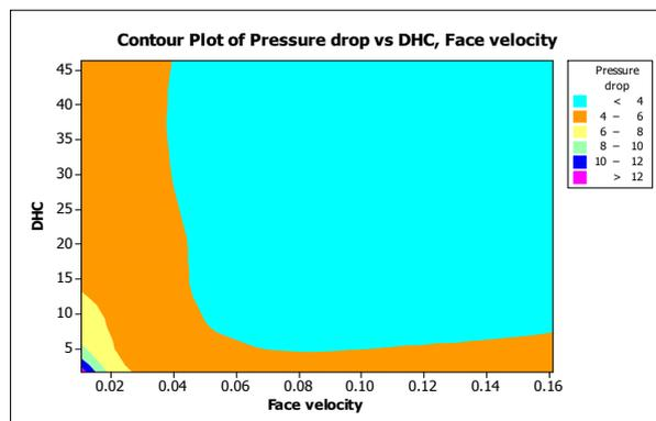
Figure 13 Contour plot of pressure drop vs. DHC & face velocity
