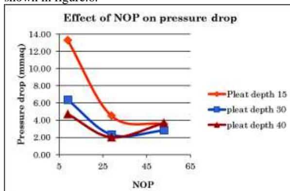
Figure 7 Effect of NOP on pressure drop
