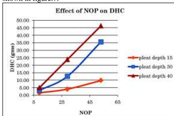
Figure 8 Effect of NOP on DHC (dust holding capacity)
